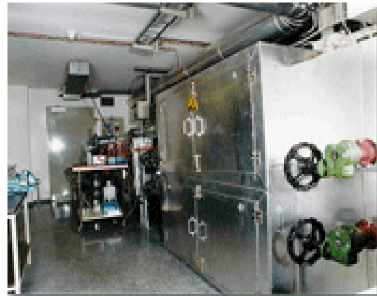
E.ON's SCR Catalyst Test Reactor
